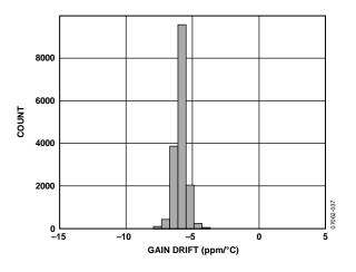
Figure 21. Gain Drift Distribution
