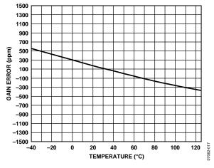
Figure 6. Typical Gain Drift
