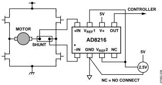
Figure 31. Motor Control Application
