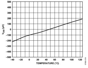
Figure 4. Typical Offset Drift
