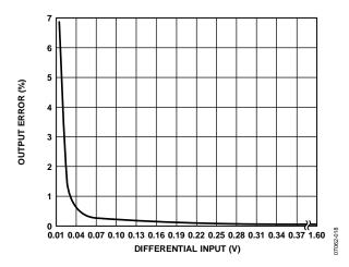
Figure 17. Output Error (%) vs. Differential Input Voltage (Unidirectional Operation (V<sub>REF</sub>1 and V<sub>REF</sub>2 Connected to GND))
