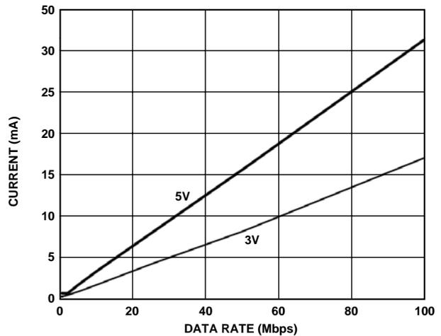
Figure 13. Typical ADuM2401 V<sub>DD1</sub> Supply Current vs. Data Rate for 5 V and 3 V Operation
