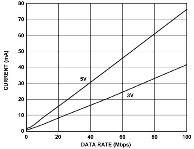
Figure 11. Typical ADuM2400 V<sub>DD1</sub> Supply Current vs. Data Rate for 5 V and 3 V Operation
