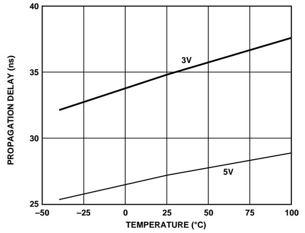
Figure 16. Propagation Delay vs. Temperature, C Grade
