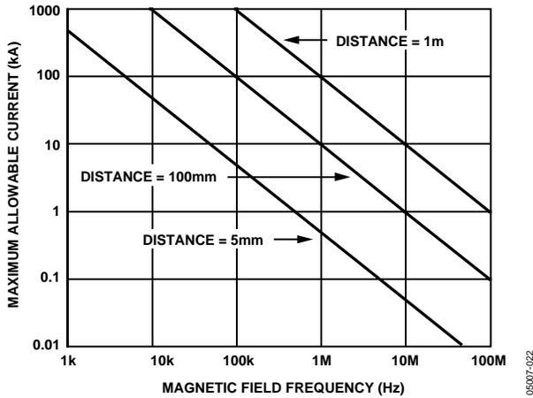
Figure 20. Maximum Allowable Current for Various Current-to-ADuM240x Spacings
