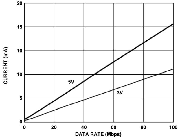
Figure 12. Typical ADuM2400 V<sub>DD2</sub> Supply Current vs. Data Rate for 5 V and 3 V Operation
