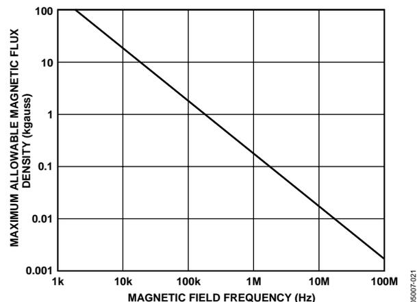
Figure 19. Maximum Allowable External Magnetic Flux Density
