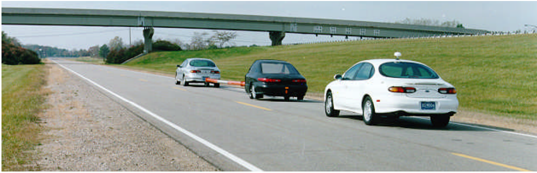
Figure 1. Surrogate target (lead vehicle) methodology employed at the General Motors Proving Ground (site of the majority of CAMP FCW research).
