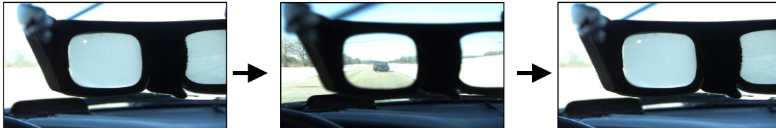
Figure 4. Time-to-collision judgment technique using occlusion glasses (1-second glimpse condition shown).
