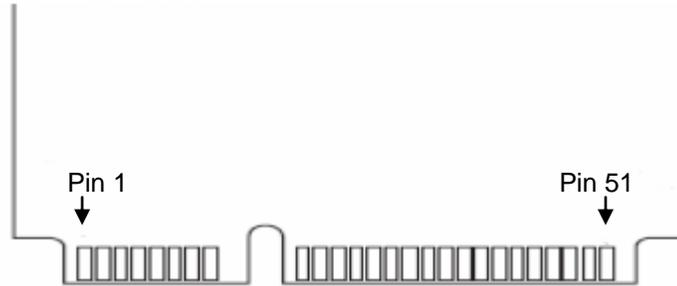
**Figure 1-2** Apacer mSATA H1-M pin assignment
