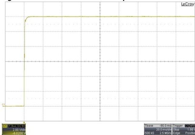
Figure 3 - Vin=40V 12V 2.5A Start Up with el load
