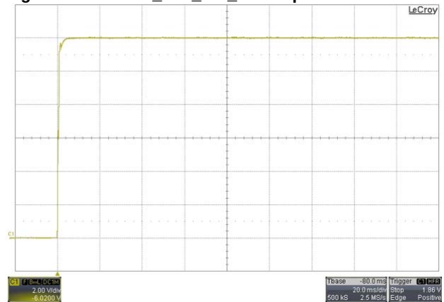
Figure 7 - Vin=57V 12V 3A Start Up
