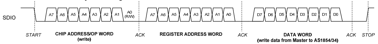
Figure 29 - I 2 C Interface Write Cycle Timing
