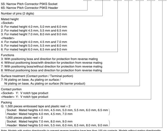
Note: Models with mating directionality to prevent reverse insertion have less than 100 pin contacts. Models without mating directionality to prevent reverse insertion have over 100 pin contacts.
