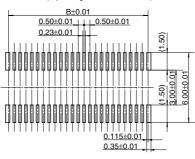
Recommended metal mask pattern Metal mask thickness: Here, 120 μm
