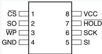
Figure 2-3. 8-UDFN (Top View)
