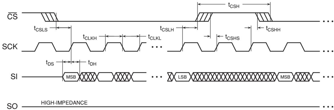
Figure 15-2. Serial Output Timing
