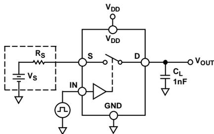
Figure 17. Charge Injection
