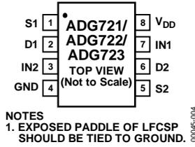
Figure 4. Pin Configuration
