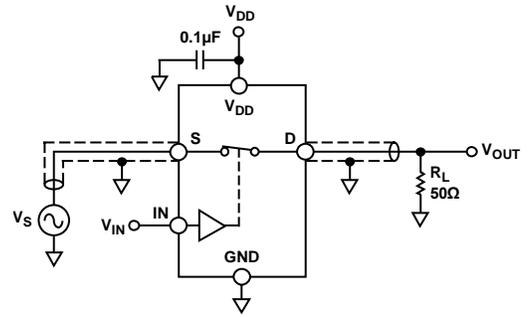
Figure 19. Channel-to-Channel Crosstalk
