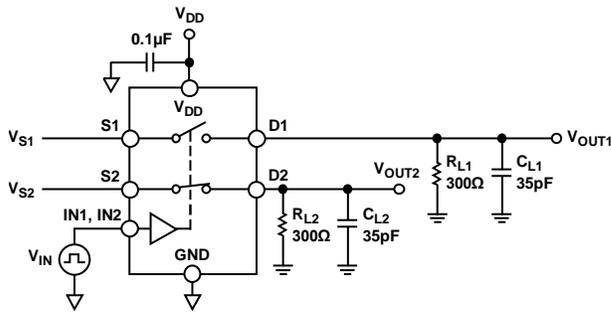
Figure 16. Break-Before-Make Time Delay,  $t_D$  (ADG723 Only)
