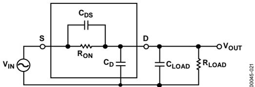
Figure 21. Switch Represented by Equivalent Parasitic Components
