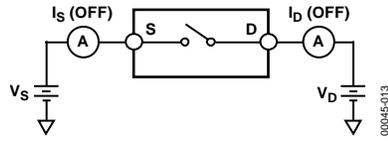
Figure 13. Off Leakage
