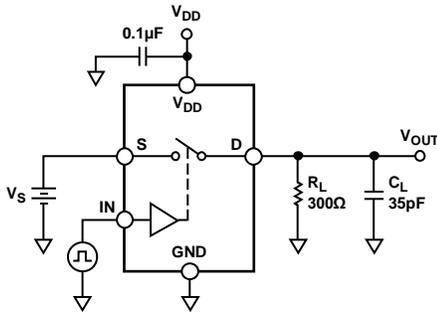
Figure 15. Switching Times
