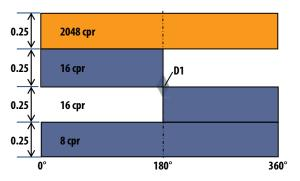
Figure 3. Code disk track 7 alignment to D1 photo detector
