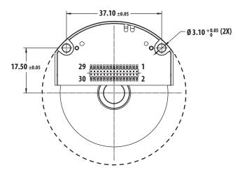
Figure 2. Alignment between read heard and the codewheel.
