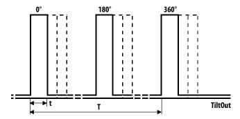
Figure 5. TiltOut signal in alignment mode.
