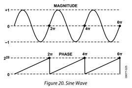
Knowing that the phase of a sine wave is linear and given a reference interval (clock period), the phase rotation for that period can be determined as follows:
