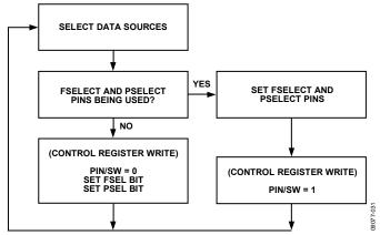
Figure 27. Flowchart for Selecting Data Sources
