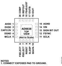
Figure 5. Pin Configuration
