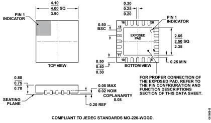
Figure 36. 20-Lead Lead Frame Chip Scale Package [LFCSP\_WQ] 4 mm × 4 mm Body, Very Very Thin Quad (CP-20-10) Dimensions shown in millimeters
