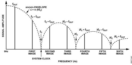
Figure 21. DAC Output Spectrum
