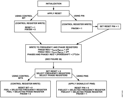
Figure 25. Flowchart for Initialization Rev. A | Page 22 of 30
