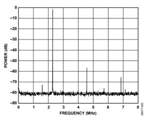
Figure 18. Power vs. Frequency,  $f_{MCLK}$  = 16 MHz,  $f_{OUT}$  = 2.28 MHz, Frequency Word = 0x2492492
