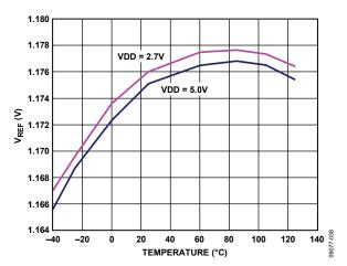
Figure 12. V<sub>REF</sub> vs. Temperature
