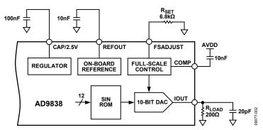
Figure 19. Test Circuit Used to Test Specifications
