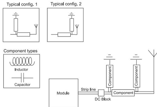
The matching network has to be individually designed using one, two or three components.
