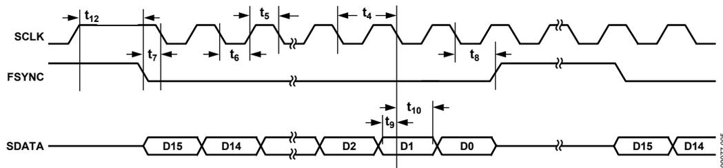
Figure 4. Serial Timing
