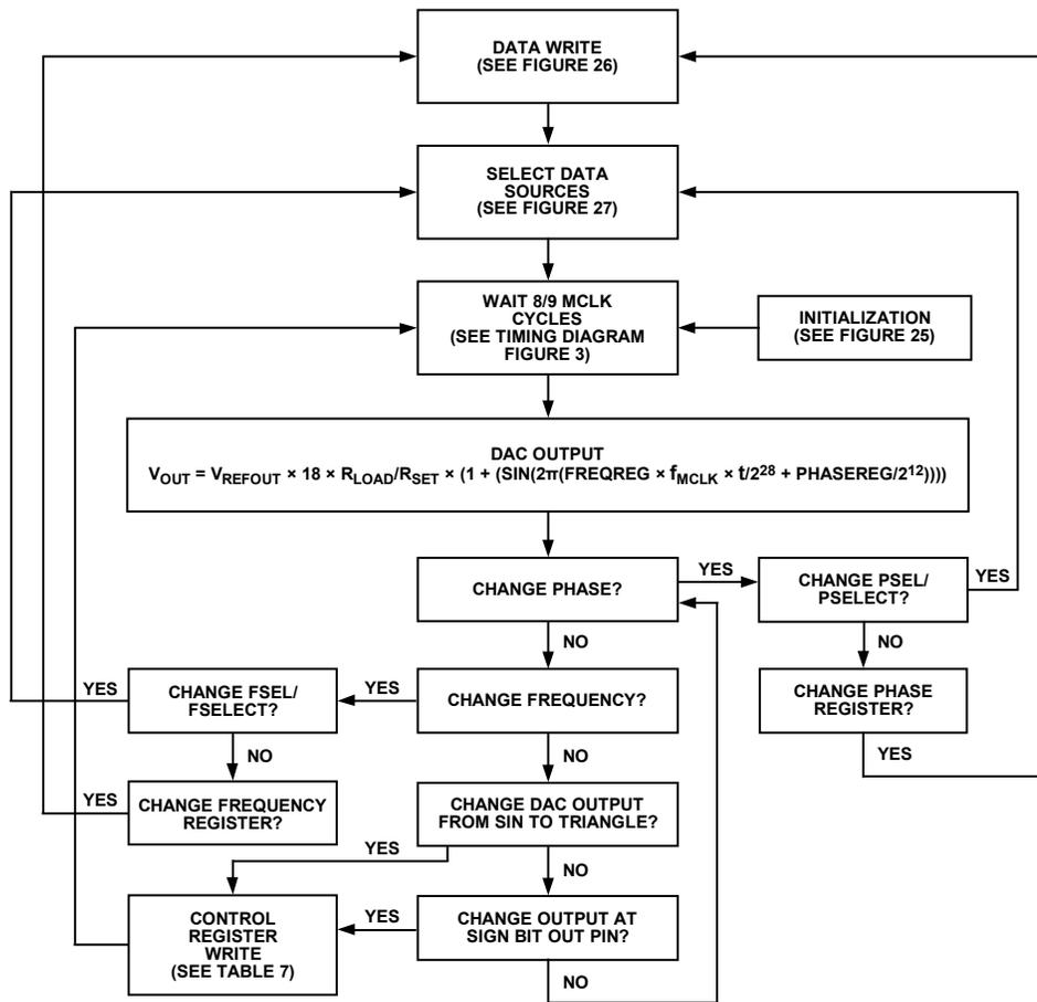
Figure 24. Flowchart for AD9838 Initialization and Operation
