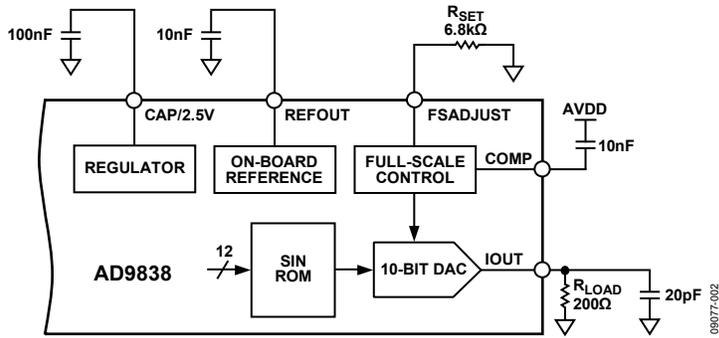
Figure 19. Test Circuit Used to Test Specifications
