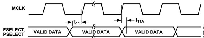
Figure 3. Control Timing
