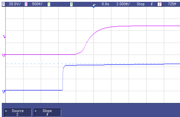
Fig.21 Typical start-up from power on of AGQ100-48S1V2
