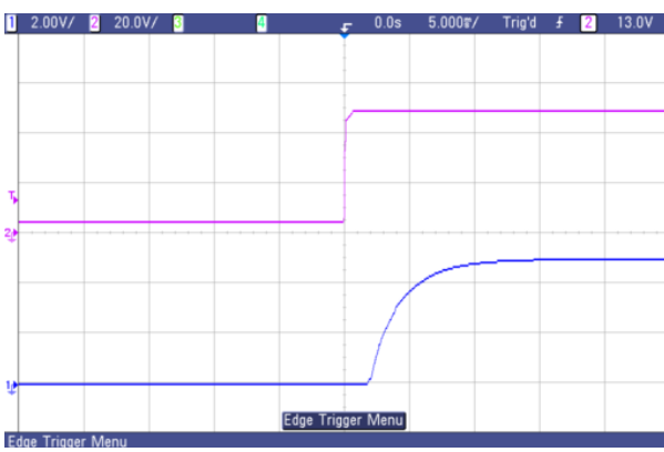
Fig.29 Typical start-up from power on of AVQ100B-48S05
