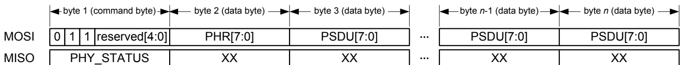
Figure 6-8. Packet Structure - Frame Write Access.
