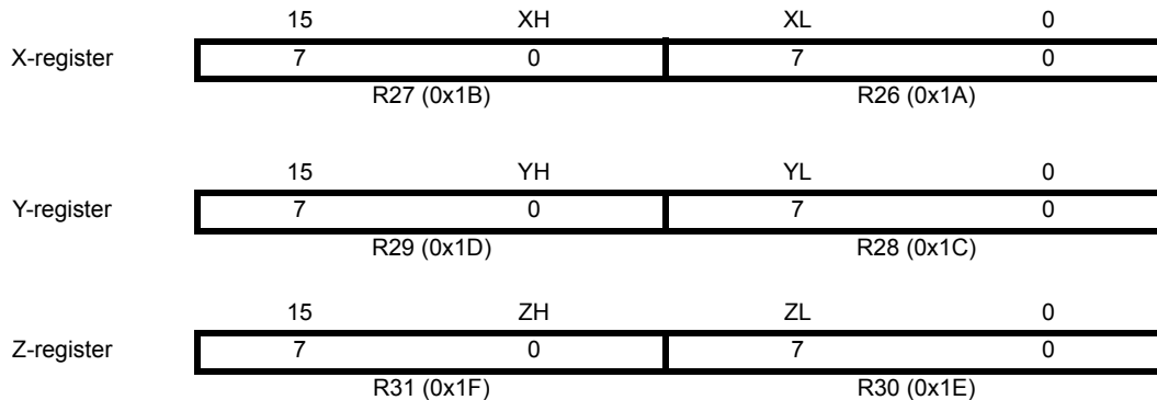
Figure 12-3. The X-, Y-, and Z-registers
